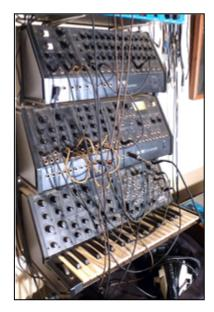
The MS-50 is a fully modular analog synthesiser featuring a single oscillator, low pass filter, ADSR and HDAR envelope generators, two voltage-controlled amplifiers, sample and hold, noise generator, inverter, integrator, divider, ring modulator, and a very useful voltage controlled modulator. For this project, the filter was not used on the MS-50, because the overall aim was to showcase the dual filter sound of the MS-20. (The character of the MS-50 filter is quite conventional by comparison.)
